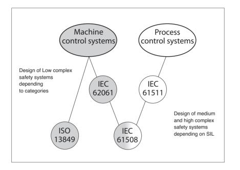
The new European Machine Directive 2006/42/EC imposes to fulfill additional safety requirements to all machines or systems delivered into the European market. The approach to define the compliance with above safety requirements refers to different standards according to the product classification:
