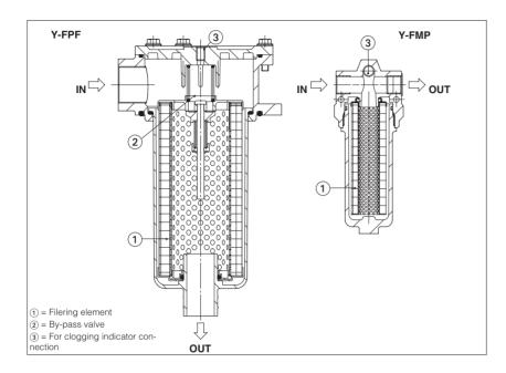
Y-FPF and Y-FMP filters have high filtering characteristics and are designed to be installed respectively on return lines and on pressure lines; they are suitable for hydraulic mineral oil or syntehetic fluids.
