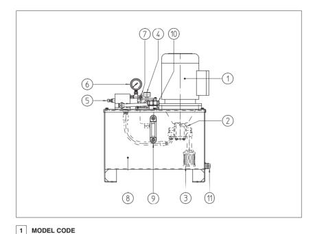
SSH hydraulic power packs are compact design standard units made according to machinery directive 2006/42/CE with vertical motor pump unit.
