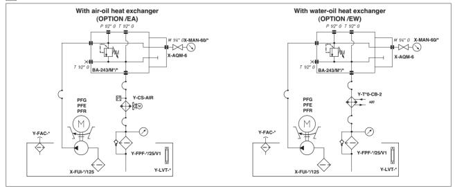
NOTE: on ASH-10 the oil filter on return line is not included and the optional mounting of heat exchanger is not available.
