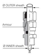
Cable glands for use with single wire armour 'W', wire braid 'X', steel tape armour 'Z', plastic insulated cables.
