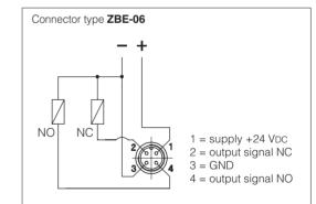
$\ensuremath{\text{NOTE:}}$  the /FV position switch are not provided with a protective earth connection
