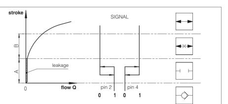
According the criteria of safety specifications, the poppet position signal must change its status inside the overlapping stroke (before the effective valve opening).
